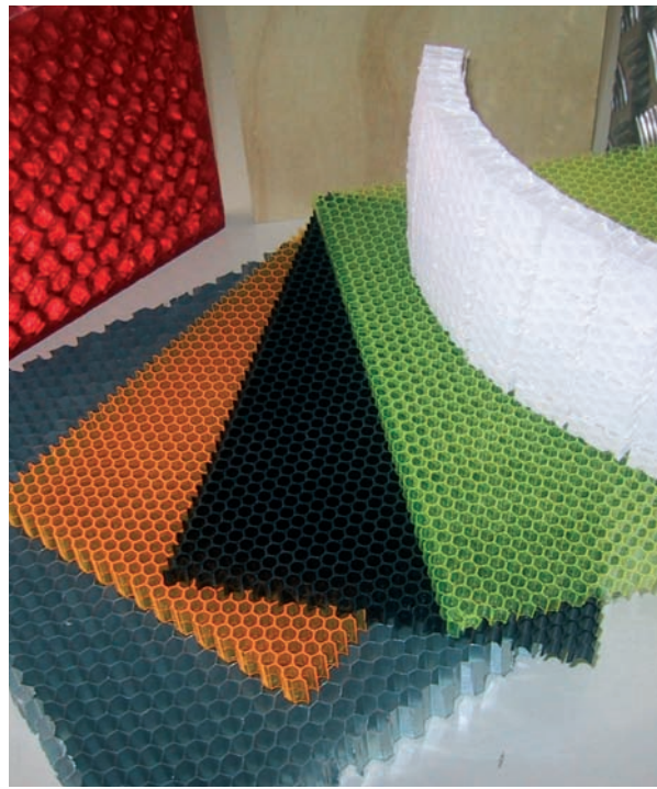
Pannelli Sandwich e alveolari d'alluminio e termoplastici Sandwich panels, aluminium and thermoplastic honeycombs
